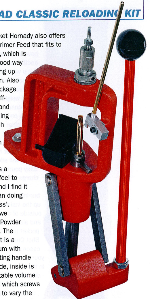
Above: The 00-7 single station press, here we see it fitted with the after market Auto Primer Feed system
